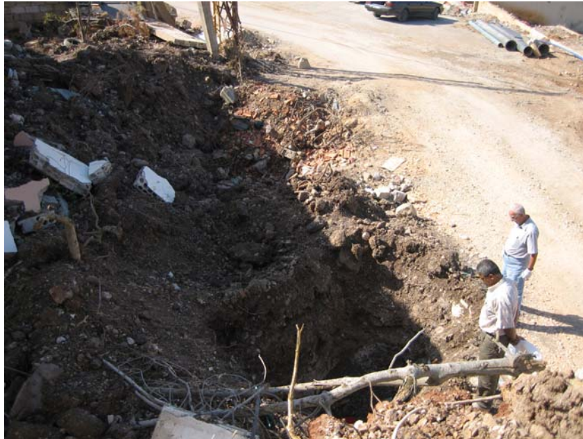
Fig 1 Crater from which sample LS6 was taken. The sample had been thrown on to a nearby roof. Geiger counter is measuring 700nSv/hr. Background in Beirut is 35nSv/hr.
